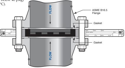
If company policy or jurisdictional regulation requires ASME Code compliance, the rupture disk devices used for pressure vessel overpressure protection shall bear the ASME Code UD symbol. The UD marking is the manufacturer's declaration that the device was manufactured in full compliance with the ASME Code.
